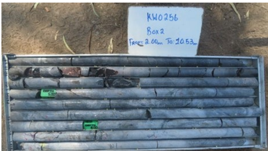
Figure 2: Shaft #1 Drill Core from Level 3 Sub-level 1 – KWO-256 — Figure 2 shows bornite and chalcopyrite occurring in highly calcified and fractured zone
