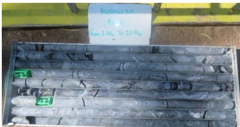
Figure 3: Shaft #1 Drill Core from Level 4 – KWO04L-319 — Figure 3 shows massive bornite with some galena in a calcitic zone.
