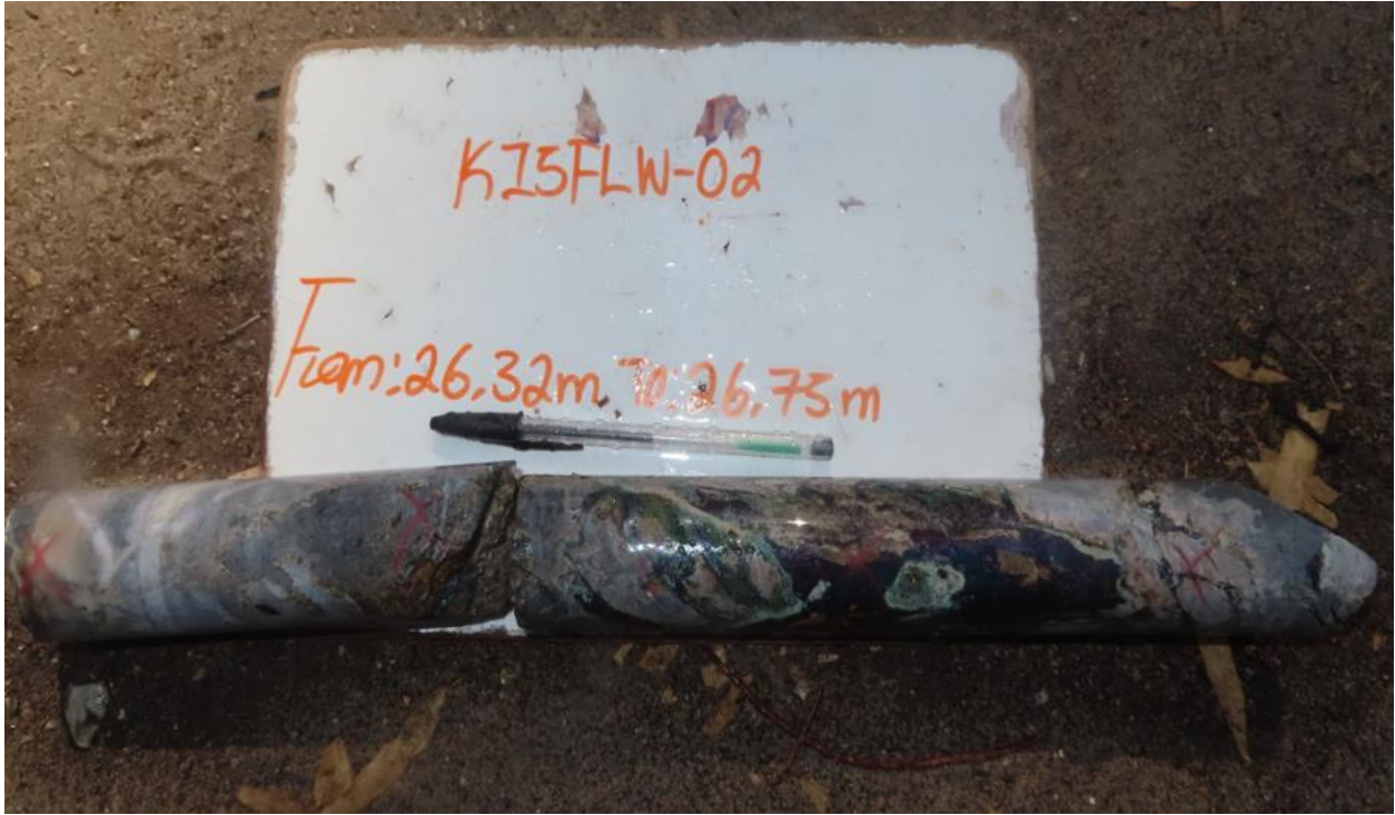
Depiction of visible copper sulfide/oxide mineralization from 26m to 35m. In weathered parts of the core, the copper is predominantly in the form of chalcocite, a copper sulfide, which the mill has proven to be effective in recovering.
