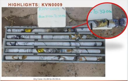
The core pictured in Figure 5, again shows shiny golden-coloured chalcopyrite mineralization (copper mineral) throughout the drill core.
