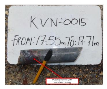
The core pictured in Figure 9 shows massive bornite mineralization with malachite coating (copper minerals) throughout the drill core.
