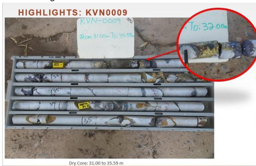
The core pictured in Figure 5, again shows shiny golden-coloured chalcopryite mineralization (copper mineral) throughout the drill core.
