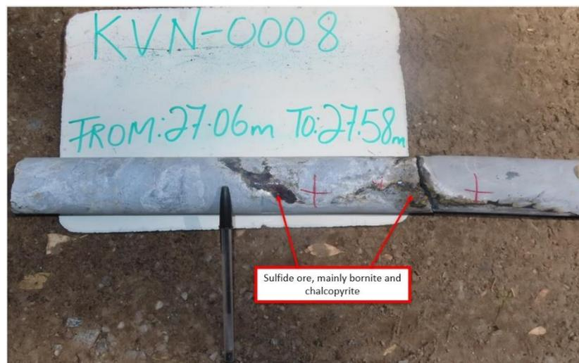
The core pictured in Figure 3 shows the clearly visible sulfide mineralization.
